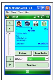
This hand held PDA computer provides the ability to remotely read meters fitted with radio transmitters. Alternatively, the device can be used for data storage where meters are read manually and the reading is input.,
